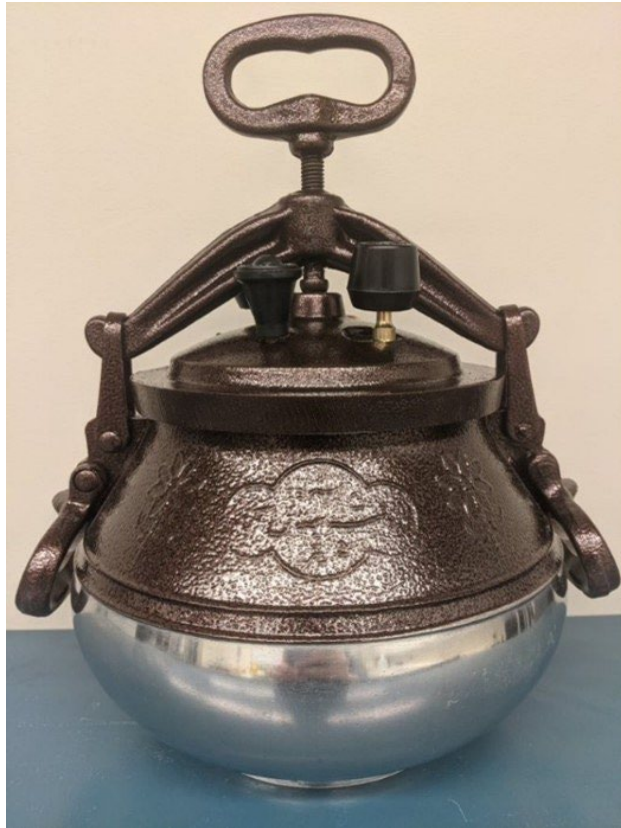
Traditional Afghan pressure cooker purchased from Etsy. Avg lead conc. 8,000 ppm (0 – 66,000 ppm).
